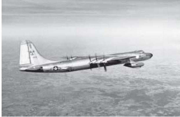
The NB-36H: The plane flew forty-seven times with an operating nuclear reactor dangling from a single hook in its mid bomb bay. Note the radiation symbol on the tail. (United
